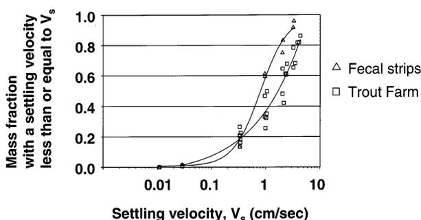
Fig. 3. Mass-based settling velocity curves.
