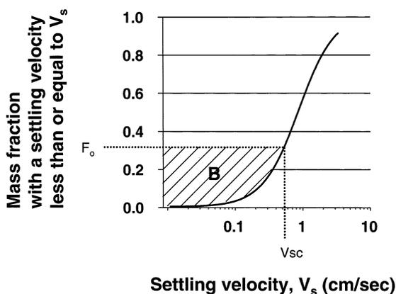
Fig. 1. A settling curve is an informative way to display settling velocity data. Refer to the text for descriptions of  $F_o$ ,  $V_{sc}$ , and  $B$ .
