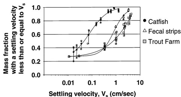
Fig. 4. Mass-based curves adjusted for the non-settleable material. Outlined symbols are data points, solid symbols are mean values, and the error bars represent the range.
