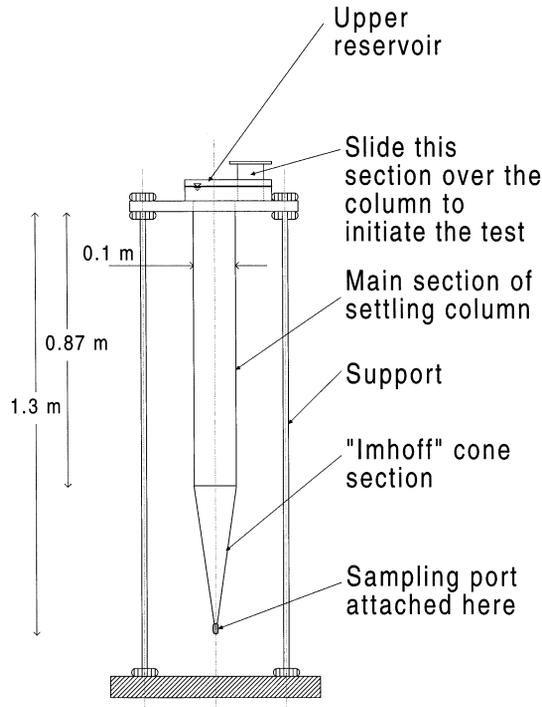
Fig. 2. A schematic of the UFT-type settling column used in this study. The column and upper reservoir were constructed of clear acrylic plastic.
