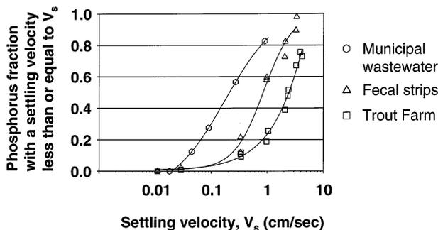
Fig. 5. Settleable phosphorus fractionated by settling velocity.
