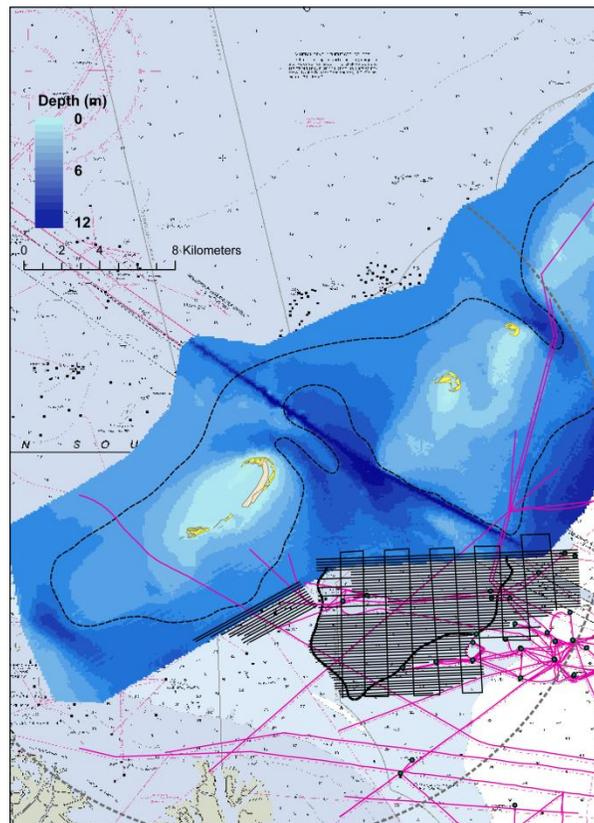
Figure 5. Offshore shoals target borrow area with proposed geophysical survey lines (black). (Pipeline infrastructure designated with pink lines.)
